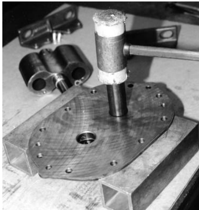
Figure 7. Tapping Bearings Out of End Plates
